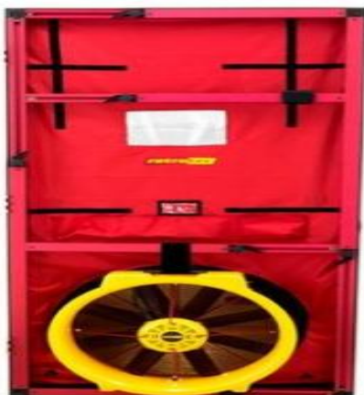
Figura 11 - Blower door system
